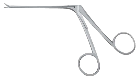
52-116-10 Shea ear forceps, scissors, straight, blade length 6.0 mm, effective length 75 mm
